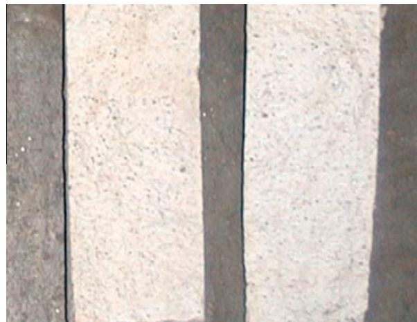
Fig. 1. Photograph of the sections of core (a length of 13 cm and a diameter of 6 cm) with open natural fractures running axially of the sample UE-7az-1770 (modified from Reimus et al. (2006)).
