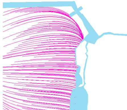
Figure 2-7 Simulated flow paths of ArcNLET after updating the waterbody polygon file
