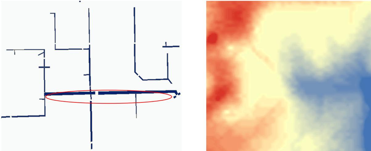
**Figure 2-1** Ditches coverage (left) and NED DEM map (right) of 1/3 Arc Second resolution. The ditches (e.g., that highlighted in the red ellipse) cannot be reflected in the DEM data.
