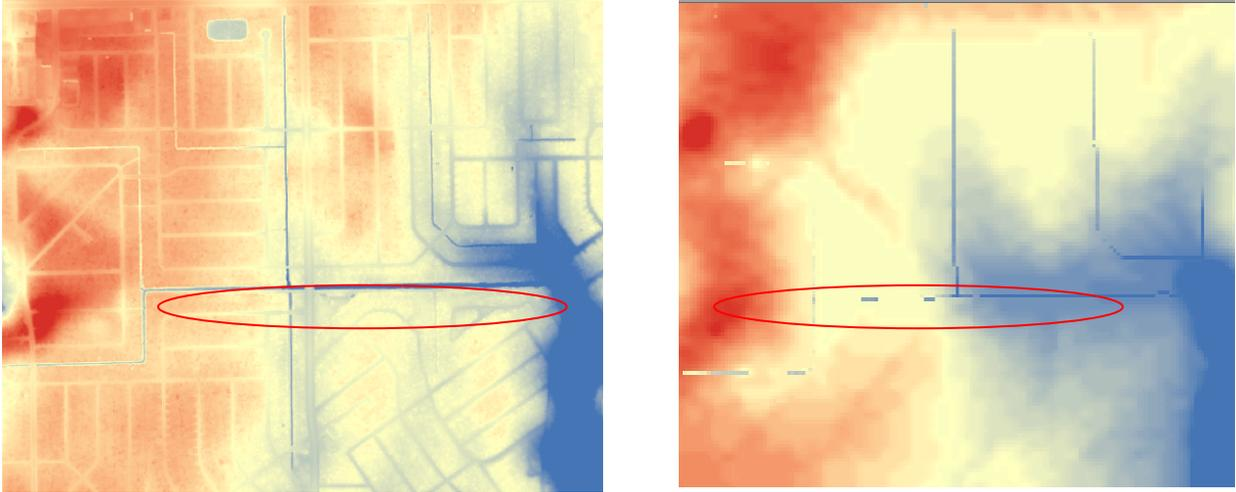
Figure 2-2 LiDAR data before (left) and after (right) re-projecting to change resolution from  $5 \times 5 \text{ ft}^2$  to  $10 \times 10 \text{ m}^2$ . The ditch highlighted in the red ellipse is preserved after the re-projecting
