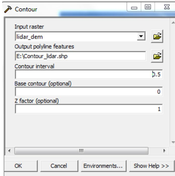
Figure 2-5 Generating elevation contour based on LiDAR DEM.
