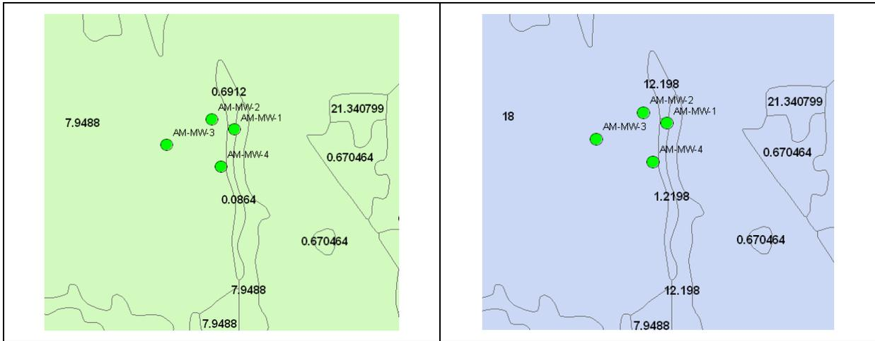
Figure 4-4 Zonal values of initial (left) and calibrated (right) hydraulic conductivity for Eggleston Heights.
