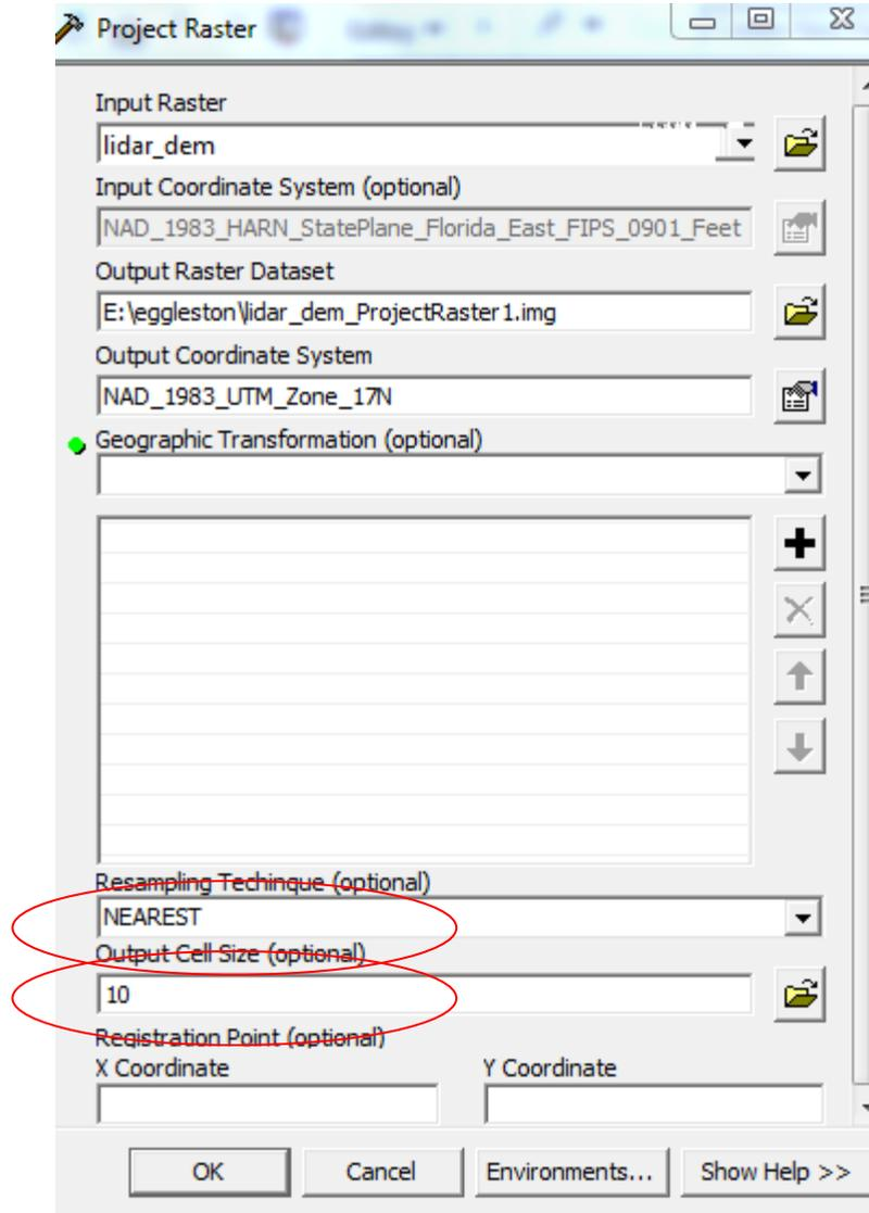
Figure 2-3 Re-projecting the LiDAR data to a coarser resolution of  $10\ 10 \times 10\ \text{m}^2$  (outpur cell size).
