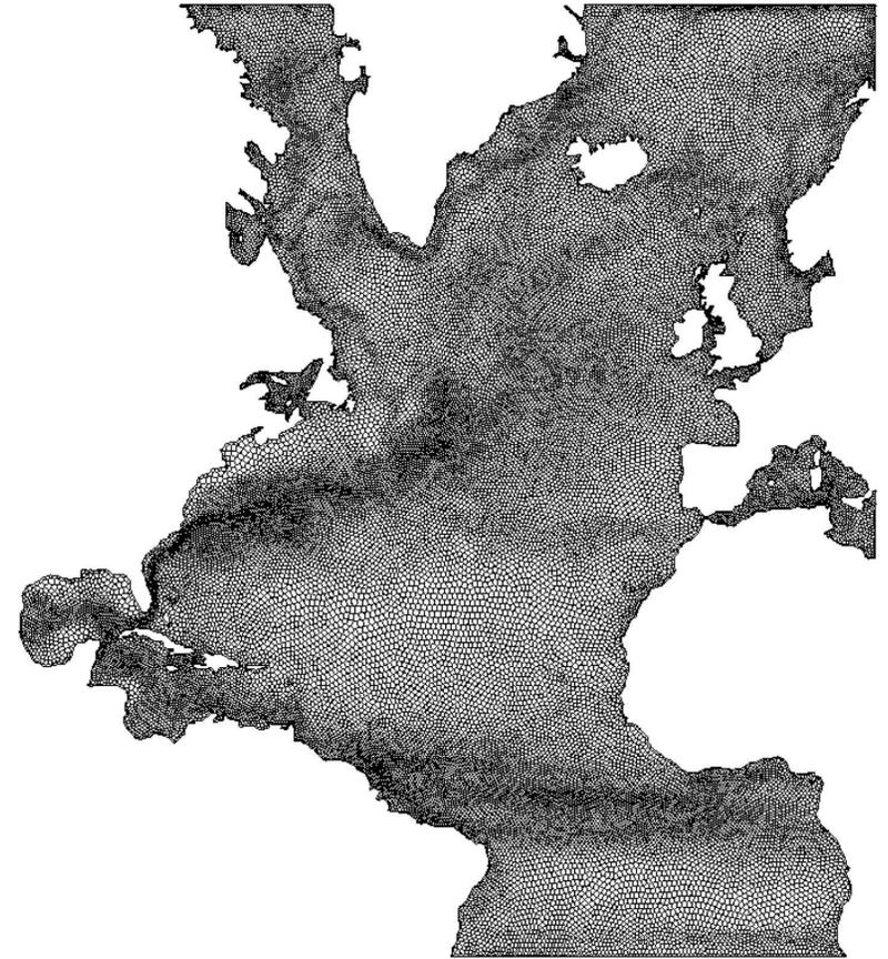
*Left: time-mean kinetic energy of the North Atlantic Ocean that is used as the CVT density function; right: a CVT mesh with 47305 nodes of the North Atlantic*
