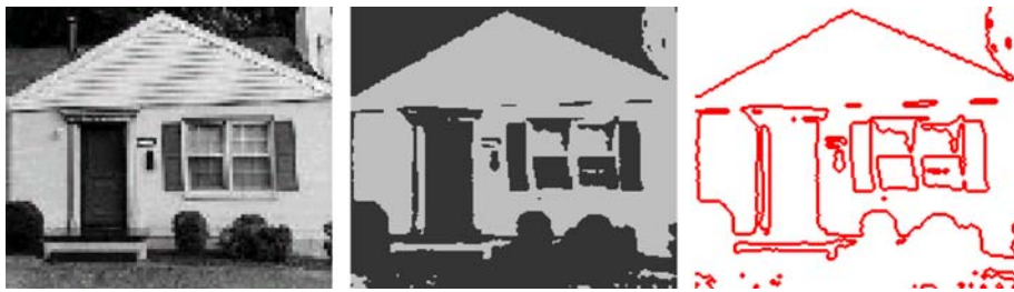
Figure 12. Left: an original grayscale image of a house. Middle: a weighted-CVT-based segmentation into two segments (with weights \lambda_\ell = |U_\ell| , i.e., \alpha = 1 ) and with subsequent averaging (with \sigma = 1.5 and \beta = 0.05 ). Right: the corresponding edges.
