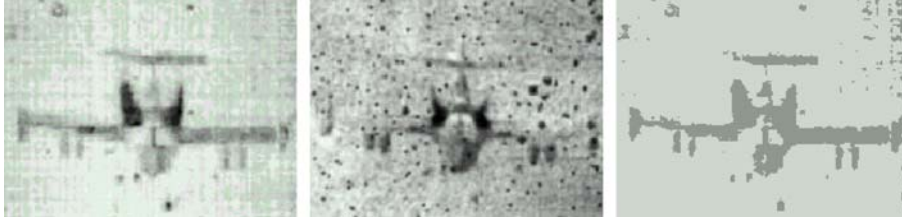
Figure 18. The left and middle images are two noisy images of an airplane. The right image is a two-color multichannel CVT approximate image using a weight v_1 = 5 for the less noisy image on the left and a weight v_2 = 1 for the more noisy image in the middle.
