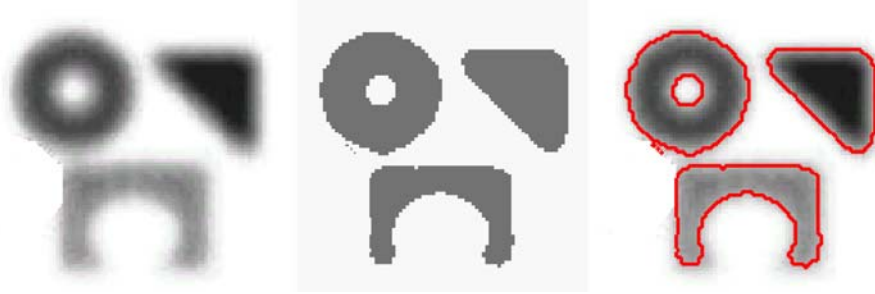
Figure 7. Left: the original image. Center: the CVT-based segmentation into two segments. Right: the edges detected via CVT-based image segmentation superimposed on the original image.
