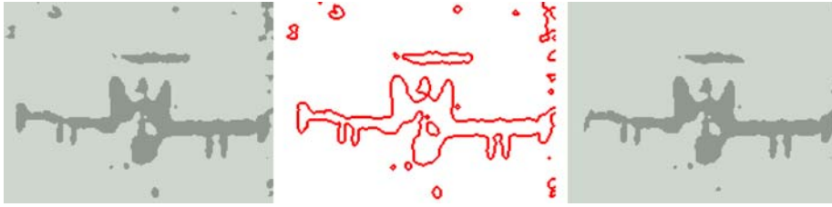
Figure 19. Multichannel CVT-image segmentation (left) and edge detection (middle) with averaging for the two-channel noisy images of Fig. 18. The channel weights are the same as that for Fig. 18, \beta = 0.05 , and \sigma = 1.5 . The image on the right is the result of filtering the image on the left.
