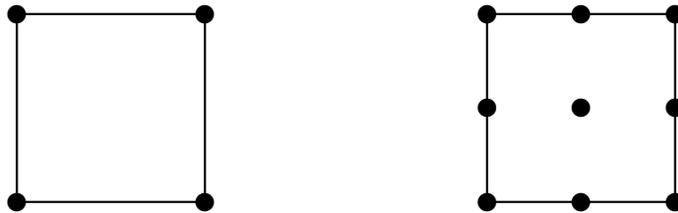
Figure 2.1: Locations of degrees of freedom for Lagrangian elements. Left: bilinear element, right : biquadratic element.
