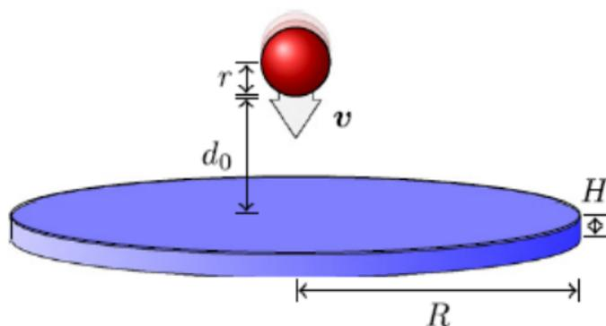
**Fig. 6.** The initial problem geometry consists of a high speed spherical projectile incident upon a cylindrical plate of the same composition.
