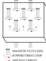
Figure 2: The set up for the numerical simulations. The magnetic field penetrates the sample as flux vortices and an applied current is transported across the sample.
