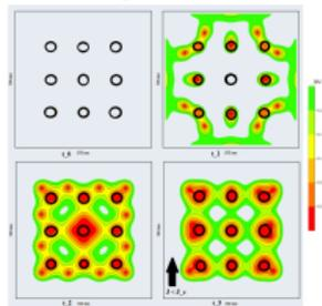
Figure 4: From top left to bottom right, vortices (red) are generated from a magnetic field. They become pinned to the normal site (black circles). When a current  $J$  is applied, the vortices remain pinned, unlike Figure 2.
