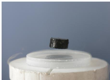
Figure : A magnet floating on top of Superconductor.
