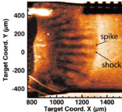
(a) An x-ray radiographic image of an experiment that used a 3D, single-mode perturbation. Time  $t = 21$  ns. Adopted from Kuranz et. al [10]
