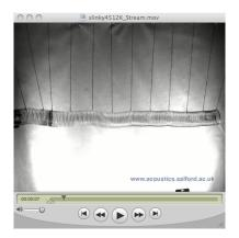
A "Slinky" is a coiled metal wire which acts like a gentle spring. Pushing it on the left, the coils compress, storing energy, and then separate, and the pressure disturbance moves to the right.
