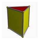
For our model, which involves 11 layers from bedrock to surface, we essentially form a stack of 10 such prisms on every triangle of the original 2D mesh.
