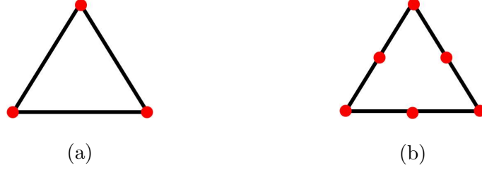
Figure 2.1: Linear and quadratic triangle elements. Figure (a) corresponds to linear pressure elements and figure (b) corresponds to quadratic elements for each component of the velocity. In all, for each triangle element there are 15 degrees of freedom.
