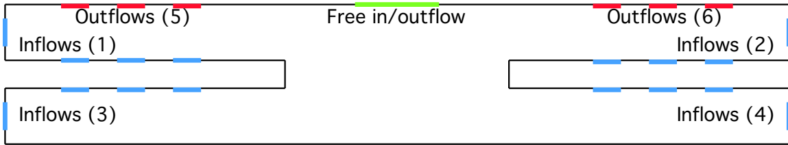
Figure 1: Prototype airline terminal with the configuration of inflow and outflow orifices.
