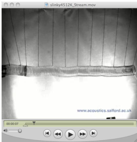
A “Slinky” is a coiled metal wire which acts like a gentle spring. Pushing it on the left, the coils compress, storing energy, and then separate, and the pressure disturbance moves to the right.
