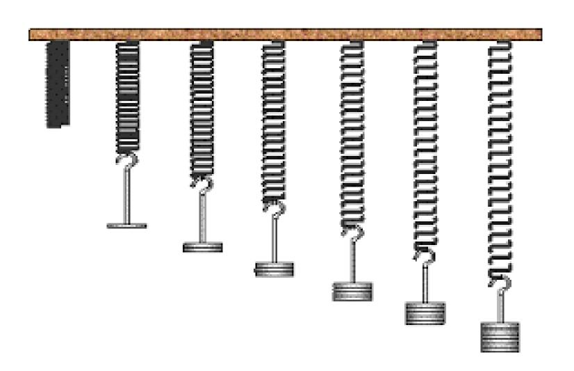
Here is sample data stored in the file hooke.csv, in which two springs were stretched by adding one more mass at a time to the end of the spring and measuring the position of the end of the spring.
