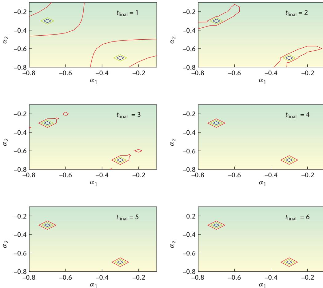
**Figure 3.** Solving problem 3. Contour plots of the residual norm as a function of the estimates of  $\alpha$  for various values of  $t_{\text{final}}$ . The contours marked are  $10^{-2}$ ,  $10^{-6}$ , and  $10^{-10}$ .
