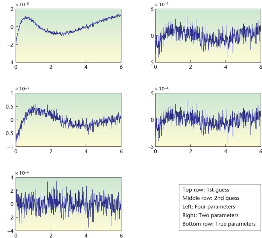
Figure 4. Solving problem 4. Residuals produced for the data with true  $\alpha = [-0.3, -0.4]$  by minimizing with two or four parameters and two initial guesses, and the residual provided by the true parameter values.
