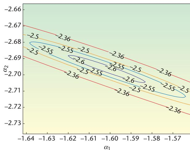
Figure 7. Solving problem 5. Contour plot of  $\log_{10}$  of the norm of the residual for various values of the  $\alpha$  parameters.
