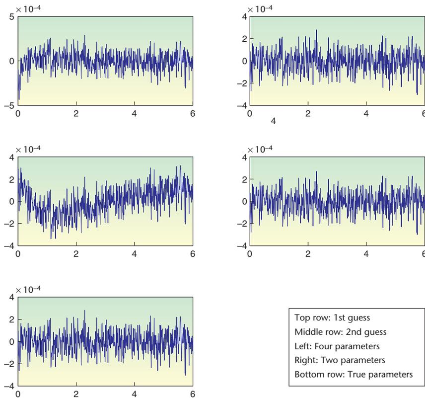
Figure 5. Solving problem 4. Residuals produced for the data with true  $\alpha = [-0.30, -0.31]$  by minimizing with two or four parameters and two initial guesses, and the residual provided by the true parameter values.
