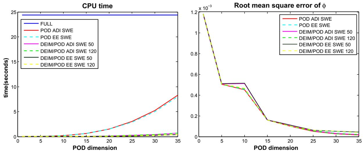
Fig. 12. CPU time of the full system, POD reduced systems and POD – DEIM reduced systems (left); Root mean square error of  $\phi$  calculated for POD/DEIM and POD reduced systems with respect to ADI FD SWE solutions.
