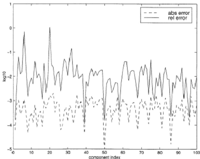
FIG. 1. The absolute (dashed line) and relative (solid line) differences between the Hessian/vector product computed with the SOA method and with the finite-difference method at the first iteration (initial guess state). The first 100 components are considered.
