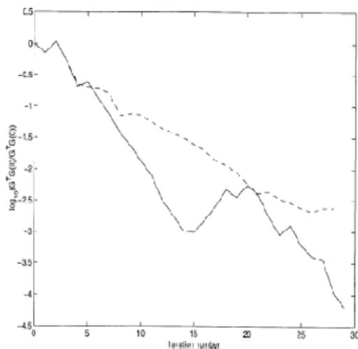
FIG. 3. The evolution of the normalized gradient norm during the minimization using the SOA method (solid line) and the finite-difference method (dashed line) to compute the Hessian/vector product.
