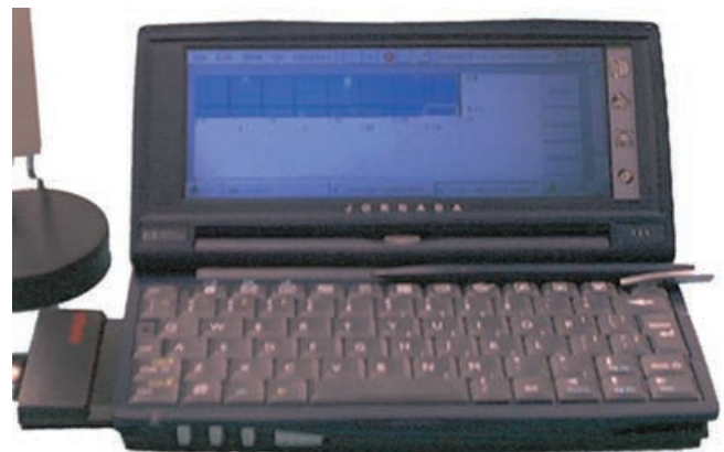
Fig. 10 Jornada 720 handheld computer. The stylus is resting at the top of the keyboard. The wireless access card protrudes on the left side of the machine. Above it is an optional external antenna
