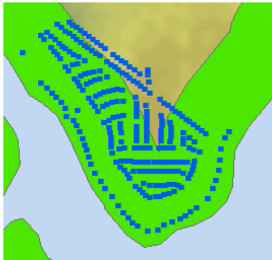
Figure 4-5. According to the empirical method developed by CDM-Smith, 223 out of 265 septic systems (blue squares) fall in the 300-meter buffer zone (green zone) and contribute nitrate to the rivers.
