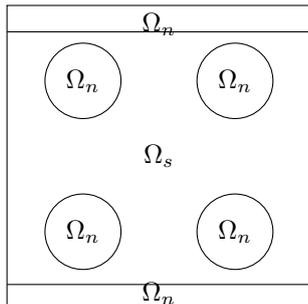
(a) A superconducting sample geometry with 4 circular normal inclusions and two metal bands at the top and bottom that serve as metal leads where an applied current enters and leaves the sample.
