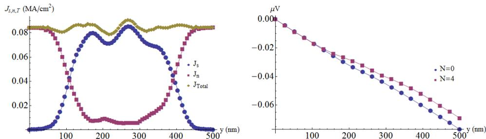
Fig. 3: The normal current, super current, and total current for the simulation after 100 time steps (left). The voltage after 10,000 time steps for the simulation with  $N = 4$  normal inclusions and for a simulation with  $N = 0$  normal inclusions. The simulation with no normal inclusions yields a larger voltage change over the domain, signifying this sample has more resistance.
