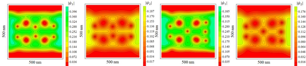
Fig. 2: The order parameters at the first time step for the MgB<sub>2</sub> parameters given in Table 1 (left pair). The order parameters after 100 time steps (right pair). The applied current has induced flux flow and distorted the vortex lattice outside of the normal inclusions.
