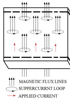
(b) The setup of the superconducting sample for the simulations. The external magnetic field  $\mathbf{H}$  is in the  $z$ -direction and the applied current density  $\mathbf{J}$  is in the  $y$ -direction. The normal metal - superconducting metal interfaces are illustrated by the dashed lines.
