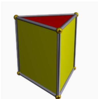
For our model, which involves 11 layers from bedrock to surface, we essentially form a stack of 10 such prisms on every triangle of the original 2D mesh.
