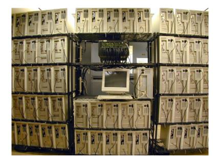
MPI (the Message Passing Interface) manages a parallel computation on a distributed memory system.
