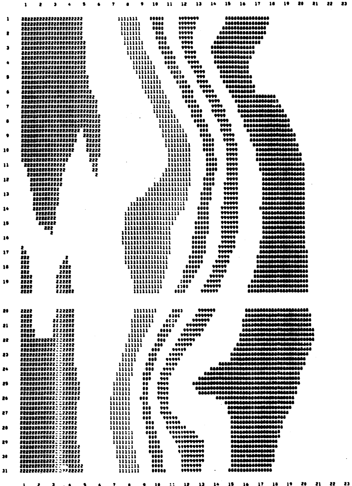
Figure 2. Height field contours after 48 hr. Space resolution \Delta x = \Delta y = 200 km; CI = 50 m; \Delta t = 1800 sec.
