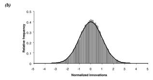
Fig. 4. Innovation vector statistics illustrated by a rank histogram of normalized innovations. The results are obtained using: (a) uncorrelated-random method, and (b) correlated-KPZ method. The solid line represents the N(0, 1) normal distribution.
