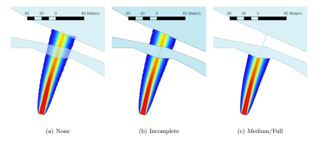
**Figure 3.14:** Example of a more complex case of post-processing on a single plume. The thin blue line represents the flow path. The light blue polygons are water bodies.
