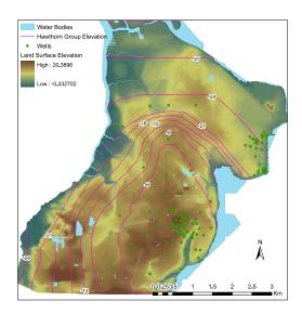
**Figure 2.7:** The locations of calibration wells in the USGS study along with a contour map of the elevation of the top of the Hawthorn group are shown on a USGS DEM with 10 by 10 m resolution. All elevation values are in meters.
