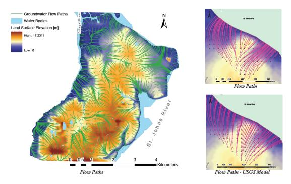
Figure 2.14: Results of running the model (with particle tracking), smoothing parameter of 50 is shown. Left: entire domain. Right: sub area located near the north east corner of the domain
