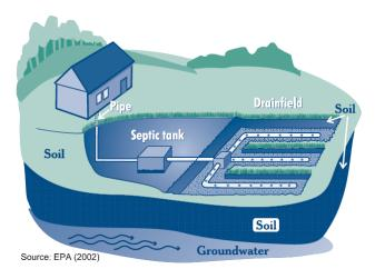
Figure 1.3: Schematic of an OWTS
