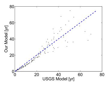
Figure 2.22: The correlation of travel time estimates between the model estimated times and the times from the USGS model of Davis et al. (1996).
