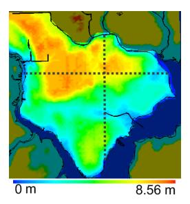
**Figure 2.12:** Model as constructed within ModelMuse. The colormap represents the elevation of the top of each cell. The highlighted area is the simulation area. The dotted lines indicate the selected cross sections of the water table used for determining recharge and conductivity parameters.
