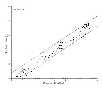
**Figure 2.8:** Simulated vs. observed head for the USGS model in the calibration wells of Figure Fig. 2.7. 121 out of the 128 well measurements fall within the 0.762 m (2.5 ft) calibration criterion (dashed lines)
