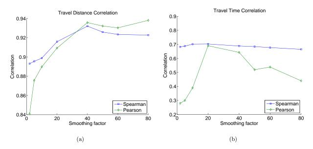
Figure 2.15: Correlation of estimated travel distance and travel time between the simplified model and the USGS model. Estimation area: entire domain
