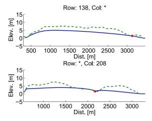
Figure 2.13: Water table and topography cross sections for the selected recharge and conductivity parameters (R=5 in/yr, K=10 ft/day). Dashed line is the topography, solid line, the water table. The dot represents the location where the water table intersects a small stream. Upper figure: east-west cross section. Lower figure: north-south cross section
