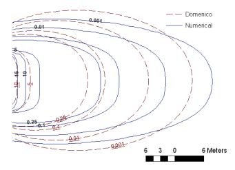
Figure 3.17: Comparison between the Domenico solution with decay,  $k = 0.008 \, day^{-1}$  and the MT3DMS solution.
