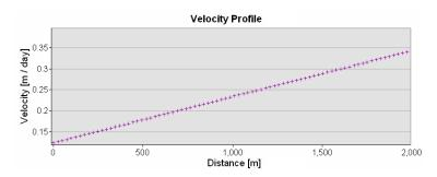
**Figure 3.18:** Velocity profile obtained using MODFLOW for testing the effect of varying velocity on the Domenico solution.
