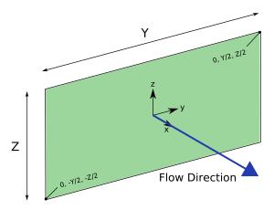
Figure 3.1: The geometry of the Domenico solution source plane.
