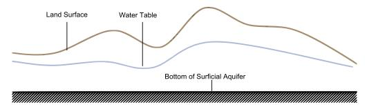
Figure 2.1: Conceptualization of the water table being a "subdued" replica of the topography.
