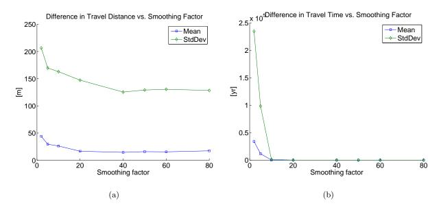
Figure 2.16: Difference between the travel distance and travel time compared with USGS model plotted against smoothing factor. Estimation area: entire domain.
