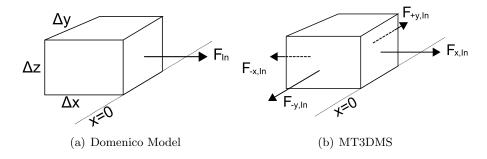
**Figure 4.4:** Source fluxes considered by our Domenico-based model compared to the ones considered by MT3DMS. The box represents a single simulation cell.
