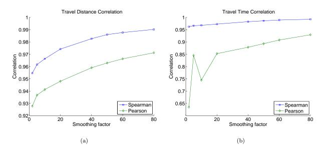
Figure 2.17: Correlation of estimated travel distance and travel time between of the model compared with the USGS model. Estimation area: sub area
