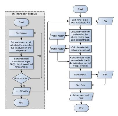
Figure 4.3: Logic flow of the denitrification module.
