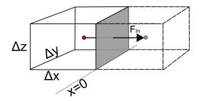
Figure 4.1: The Domenico source plane (shaded area) interpreted as the side of a simulation cell.
