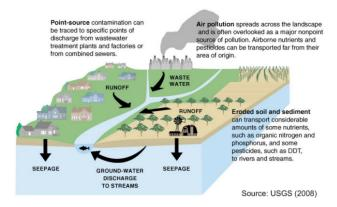
Figure 1.1: Sources of groundwater contamination.
