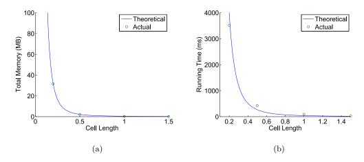
Figure 3.3: For a 3D test hemisphere, both the running time and memory requirements scale as  $O(\Delta \ell^{-3})$ , where  $\ell$  is the length of the side of the evaluation cell. This shows the benefits of evaluating the Domenico solution in 2D
