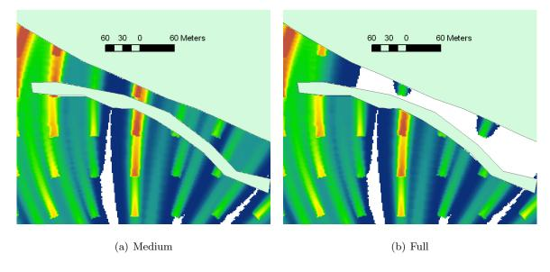
**Figure 3.15:** Example of a more complex case of post-processing with multiple plumes. For clarity, flow paths are not shown however the direction of flow is the same as in Fig. 3.13 (approx. south to north).
