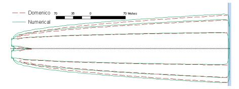
**Figure 3.22:** 0.1 and 0.01 mg/l contours for the overlapping case. No decay. The dotted line represents the cross-section of Fig. 3.23
