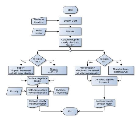
Figure 2.4: Logic flow for the groundwater flow model.
