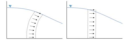
**Figure 2.2:** Illustration of the Dupuit approximation. The left figure shows flow lines with vertical gradients. The right shows flow under the Dupuit approximation. Dashed lines represent equipotentials and arrows represent flow direction. The solid line represents the water table.
