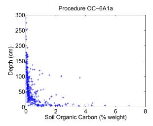
Figure 3.27: Soil depth plotted against percent organic carbon at that depth for soils in Florida. Data Source: USDA Natural Resources Conservation Service (http://ssldata.nrcs.usda.gov). Procedure 6A1a is described in detail in the NRCS Soil Survey Laboratory Methods Manual (U.S. Department of Agriculture, 2004)
