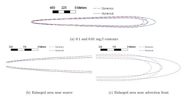
Figure 3.19: Comparison of Domenico and MT3DMS plumes for a spatially varying velocity.
